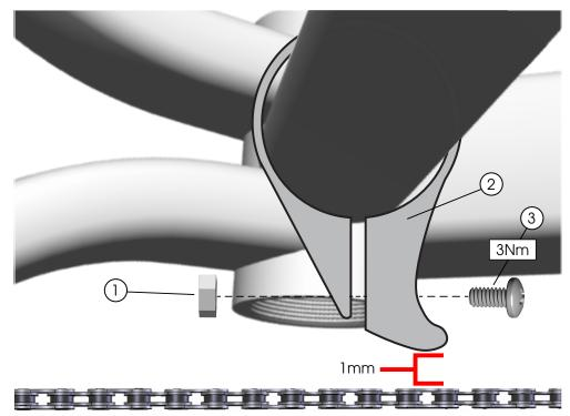
Rotate the chainkeeper as necessary so there is 1mm of clearance to the chain.
